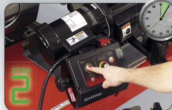
Compensate lateral runout with single-point adjustment.
